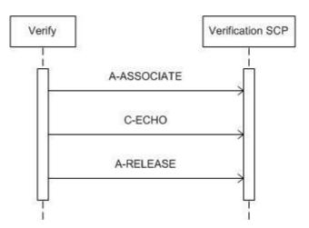
Figure 6: Data Flow Diagram - Verification as SCU
