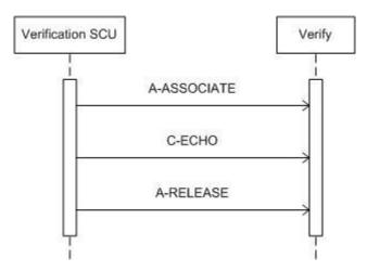
Figure 4: Data Flow Diagram - Verify
